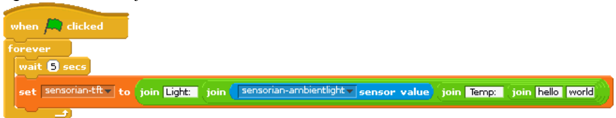
Figure 18: Setting the left side of the new join block to "Temp: " and adding another join block into the right side
