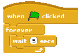
Figure 13: Add a wait block to control the refresh rate of the main loop
