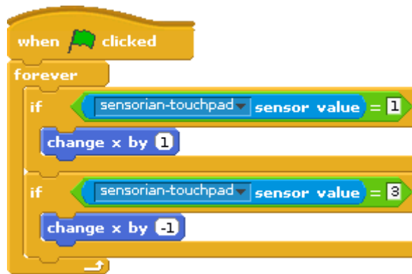
Figure 6: The final program. The car moves along the horizontal axis based on the capacitive touch button that is pressed
