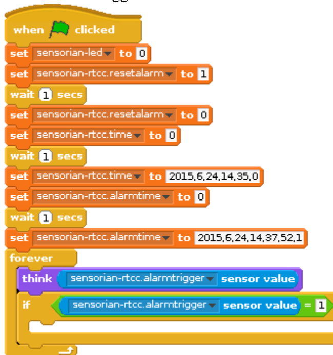
Figure 40: Using an if block to run code if the alarm is triggered
