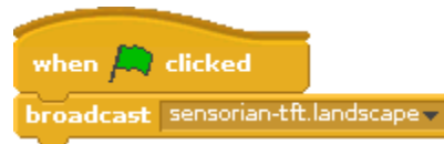
Figure 27: Broadcast "sensorian-tft.landscape" to make the TFT-LCD display text in landscape (wide) mode
