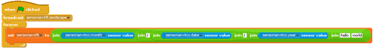
Figure 34: Adding the sensor value and join blocks
