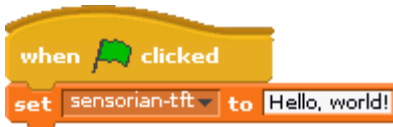
Figure 2: The final program which simply prints "Hello, world!" on the TFT LCD
