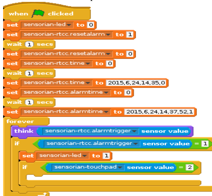
Figure 42: Add an if block to run code if B2 is pressed while the alarm is triggered
