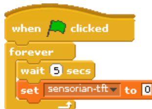
Figure 14: Add this set block to clear the TFT-LCD
